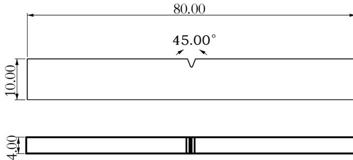
Impact testing specimen; ASTM D256 (ISO 179, GB/T 1043)
